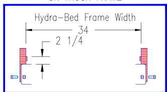
Place front FLL-2 approx 3 1/2" from cab. Drill 5/8" hole in frame of truck and bolt strap in place. Place 2x2x2 1/4" tubular block on truck frame against inside of strap.
